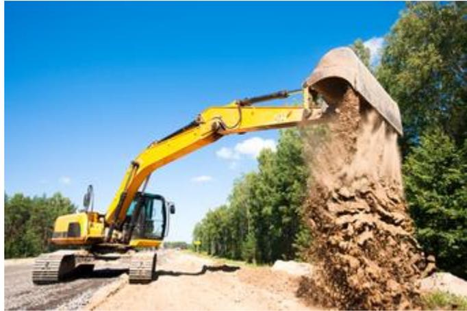
Bucket capacity impacts how much material can be removed at any one time. For large excavation projects, time is critical. However, for more precise projects, a smaller bucket capacity allows for consistent operation. Bucket capacity does not have a large impact on price as different types and sizes of buckets are available as accessories.
