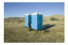
Such units are larger, can serve up to 125 people and are pulled behind trucks similar in size and shape to a horse trailer or camper. They have steps and handrails for access to the facilities, water tanks, and waste disposal features so they can be emptied at a dump station.
