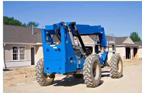
Newly redesigned to incorporate the latest ergonomic features like tiltable steering wheels, many telehandlers also feature cab designs that are roomy and comfortable. This enables longer, more productive work shifts by minimizing fatigue and repetitive stress injuries. Most rough terrain forklifts within this range are run by a single joystick that controls all boom functions and hydraulics for simple and efficient operation.
