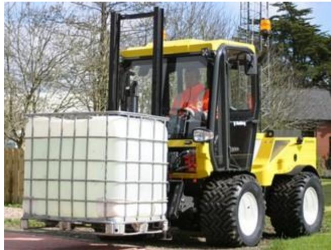
Most lifts in this category come with two-wheel and four-wheel drive. And depending on the model selected and your intended application and work environment, straight mast forklifts can be powered by diesel fuel or propane. This enables them to be used outdoors as well as indoors.
