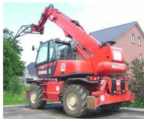
Also employing joystick controls, some machines offer the addition of a second joystick on the left side of the machine to operate rotation separately. Four-wheel, power assisted steering is common among leading brands as is minimized slip differential on the rear axle to boost traction and safety.
