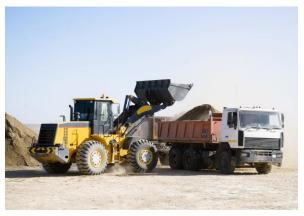
example). It does not represent the total lift capacity. On average, you can expect to find breakout force ranging between 9,000 to 47,000 lbs.
