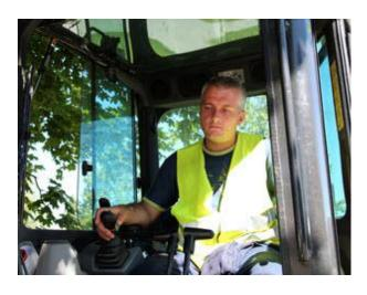
pedals, requiring both hands and feet. This led to operator fatigue, injury, errors, and ineffective overall use of the machinery. With the joysticks, all controls are on two levers. The left hand controls the swing and extension of the stick while the right controls the bucket and boom. Joystick also use roller pads for the thumb as well as push buttons for functions.
